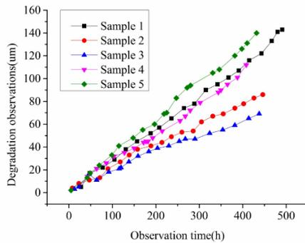
Fig. 1. Machining accuracy degradation paths.
