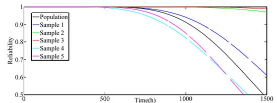
Fig. 5. Reliability of the CNC machine tools with informative prior distribution.
